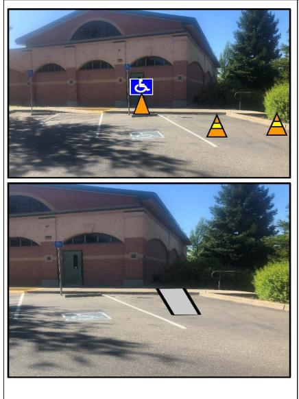
The existing van accessible space/access aisle is not accessible for voters using the library entrance because the path of travel will not allow a wheelchair to use the sidewalk for entry when the library door is open.
