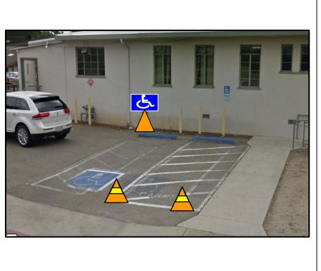
The accessible parking and access aisle is not clearly marked and there is no designated van accessible sign.
